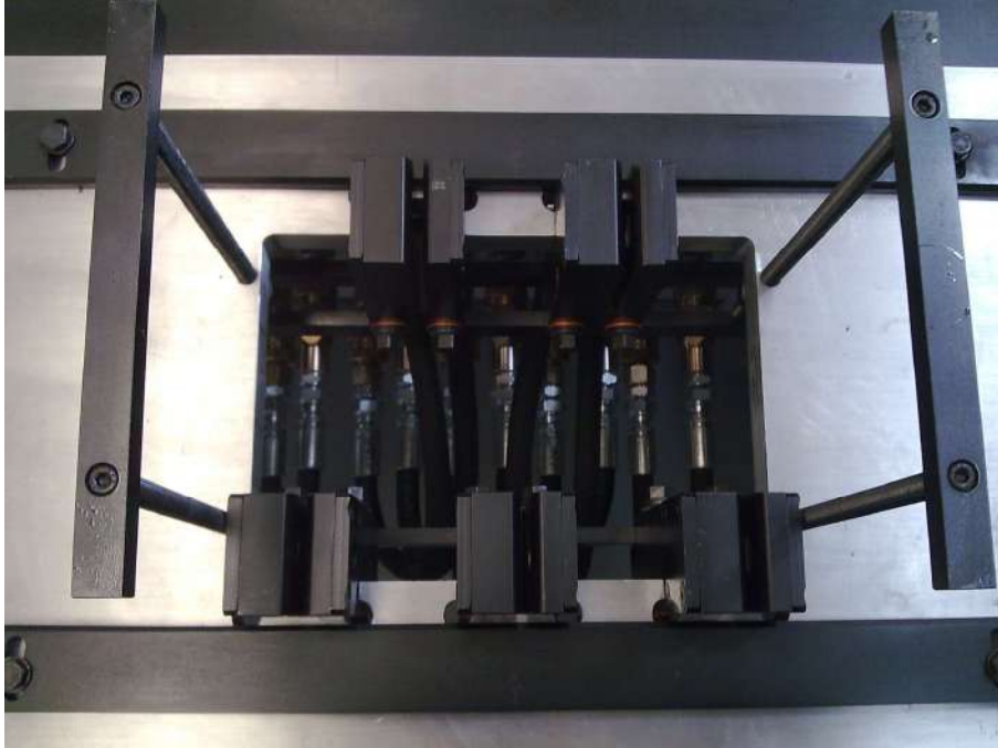
Sample of punching set 6x1 for car batteries.
