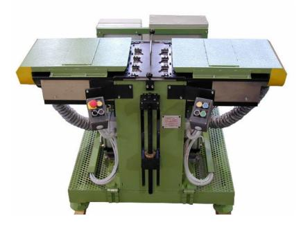
The IGM machine is designed to weld the groups used for industrial elements production and it has been developed during many years of experience in this field. The best-known battery manufacturers use this model.
